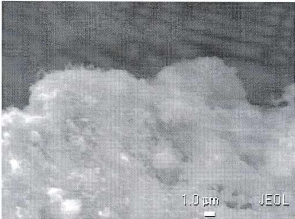
Fig. 3. Image of nanotubes in scanning microscopy mode. Magnification  $2.5 \times 10^3$
