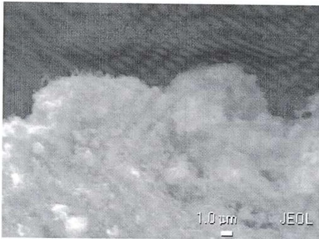
Fig. 5. Image of nanotubes in scanning microscopy mode. Magnification  $5 \cdot 10^5$
