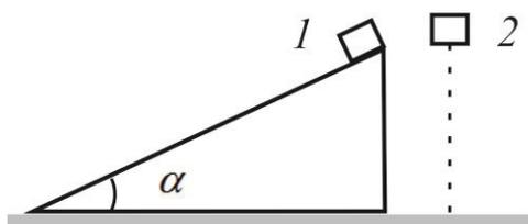
$$\left[ v_1 = v_2 = \sqrt{2gh}; t_1 = t_2 \cdot \sin \alpha \right]$$
