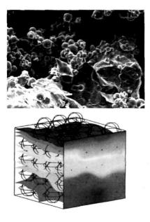
Fig.1: (left) SEM of the sintered layer reveals a hierarchical type of morphology. (right) Modeling of heat transport in a porous powder layer showed high inhomogenity of the temperature field in a mixture of particles of different sizes.
